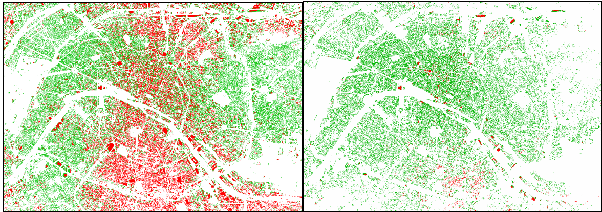
Figure 12: coverage map at the ground-floor (left) and fifth floor (right) levels for the SFN configuration with reception diversity; the receiver threshold is -73 dBm; the green areas are covered; the red ones are not covered.
